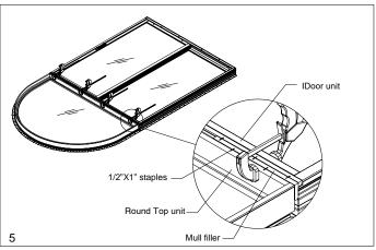
7. Center and attach mulling tin over mullion 3/8" (10) from the interior and fasten with 1/2" x 1/2" staples to jamb of round top unit. Measure and pre-drill screw locations with a 7/64" drill bit through the first layer of the patio door Ultrex jamb as shown. Attach with #8 x 3/8" pan head screws. Finish fastening the mull tin with 1/2" x 1/2" staples on the wood jamb liner of the patio door unit. See illustration 6.
