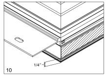
Position units together in the desired configuration. Check to be sure that the frames at both ends of the mullion are flush and the nailing fin kerfs are aligned. Lightly clamp units together on interior (use wood blocks to protect interior) near each end to hold mulled units in place. See illustration 11.
