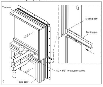
Center mulling tin over mullion and attach to wood jamb liner with 1/2" x 1/2" 16 gauge staples. Follow location and quantity recommendations for staples shown in illustration 7. Measure 3 1/8" (79) from the exterior edge of the jamb and predrill screw locations through mulling tin and first layer of the patio door Ultrex using a 7/64" drill bit. Attach tin to Ultrex with #8 x 3/8" Phillips panhead wood screws. See illustration 7.
