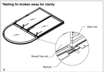
6. Making sure the mulled units are flush at the interior and square on the ends, fasten the interior of mulled units with 1/2" x 1" staples spaced every 4" (102). See illustration 5.
