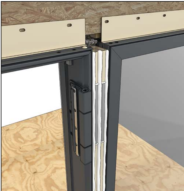
Figure 268 Show sealant with aluminum fillers and vinyl.
