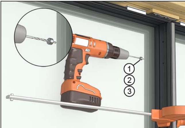
Figure 198 Use stop collar to determine depth. See table below
