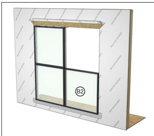
Figure 53 Install B2 (exterior view)
