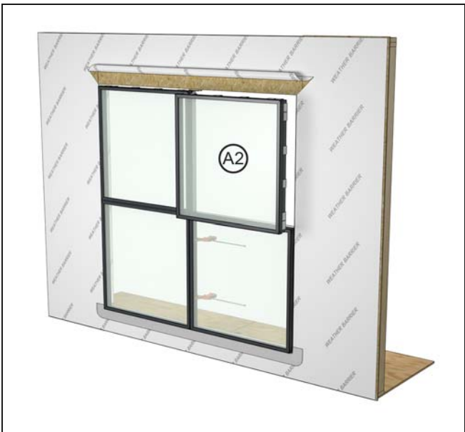
Figure 59 Install the A2 (exterior view)
