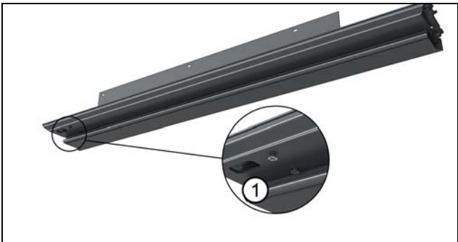
Figure 213 Outswing X Head jamb: the head jamb strike fasteners are installed from the factory. The support strike is fastened
