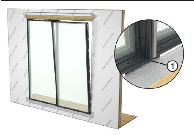
Figure 22 Set second unit and align frames (inset)
