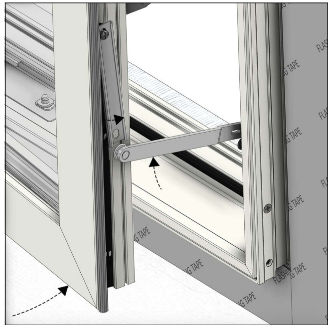
Figure 11 Inserting Limiter Arm
