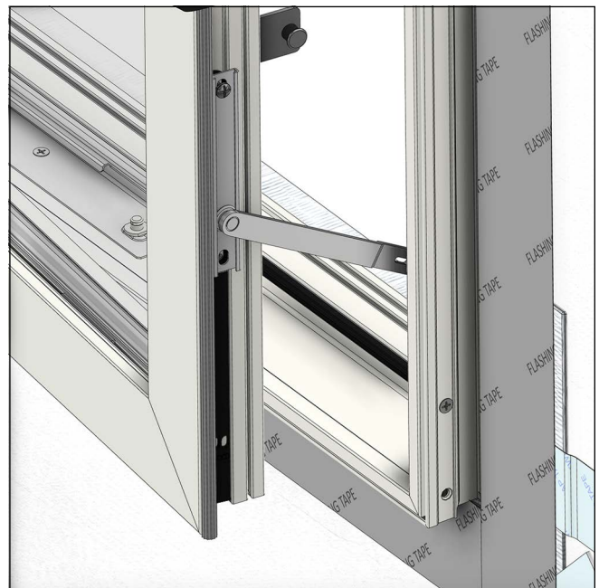
Figure 12 Inserting Limiter Arm
