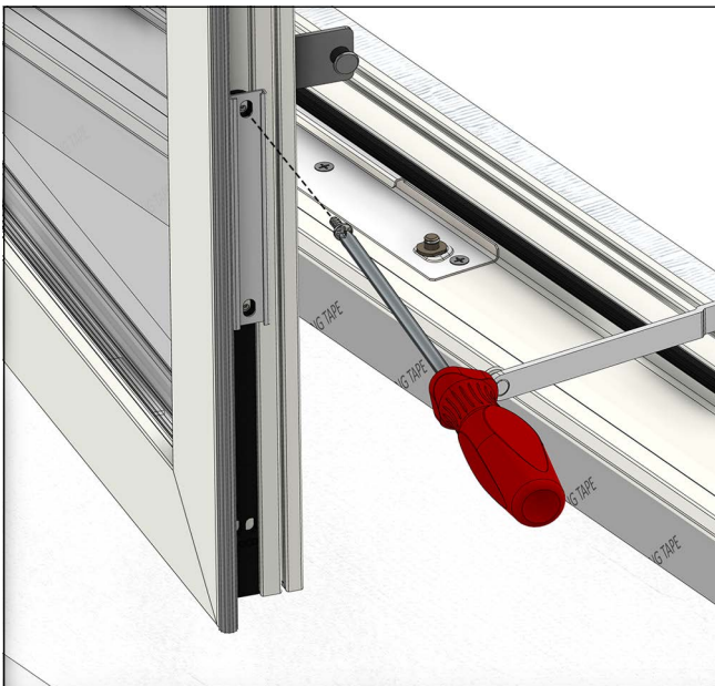
Figure 10 Installing Top Screw
