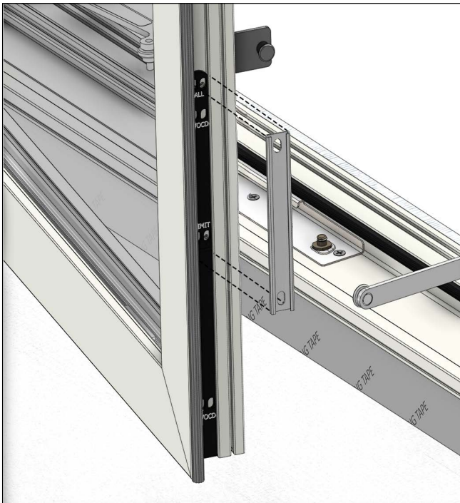
Figure 9 Lining Up Track
