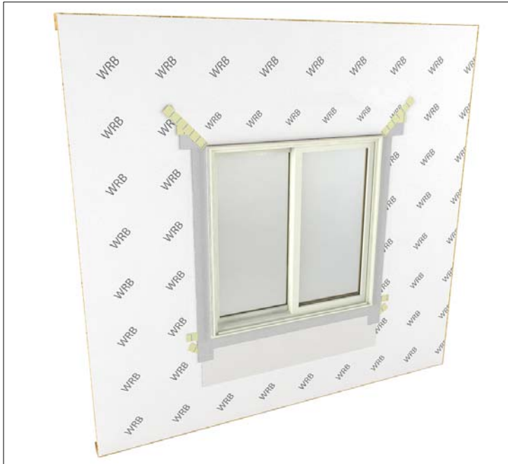
Figure 13: Sealing the installation in air barrier applications.
