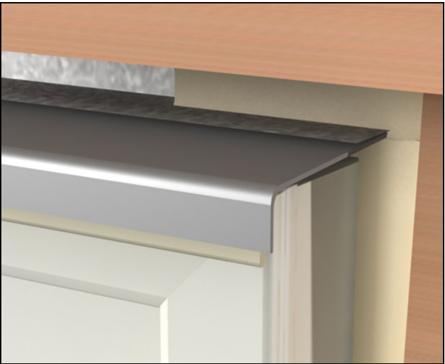
Figure 45 Apply sealant between window and exterior finish.
