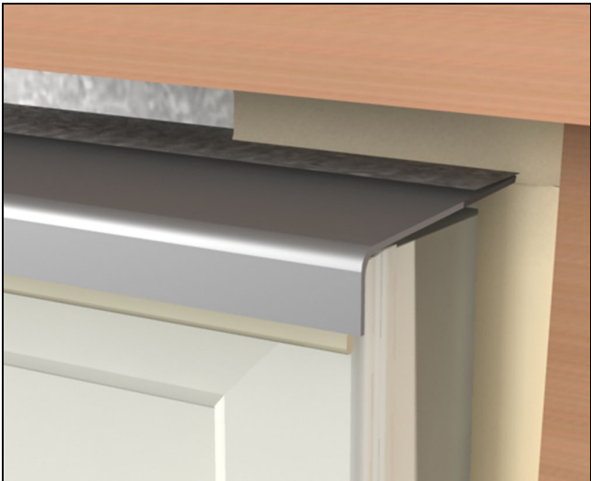
Figure 47 Apply sealant between window and exterior finish at head jamb.
