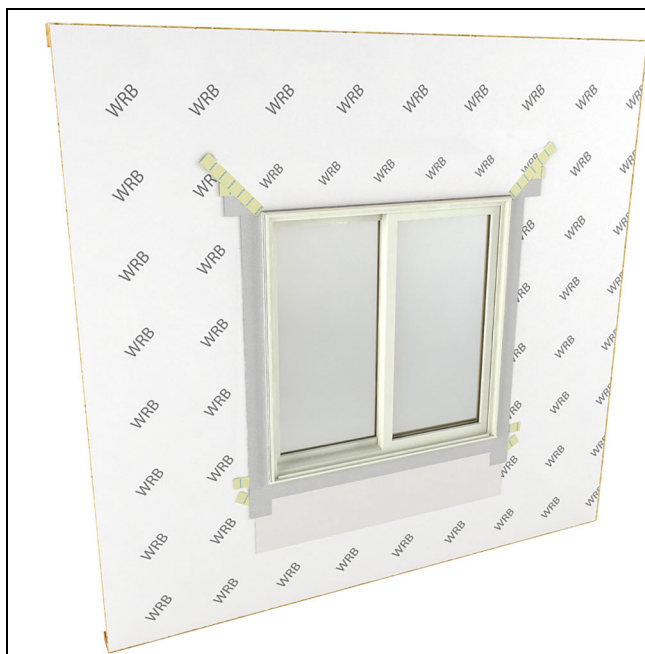
Figure 42 Sealing the Installation in air barrier applications.
