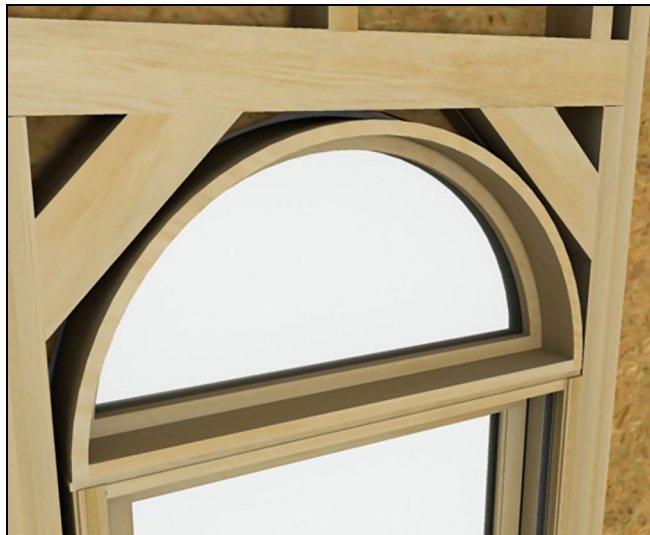
Figure 2 Typical rough opening.
