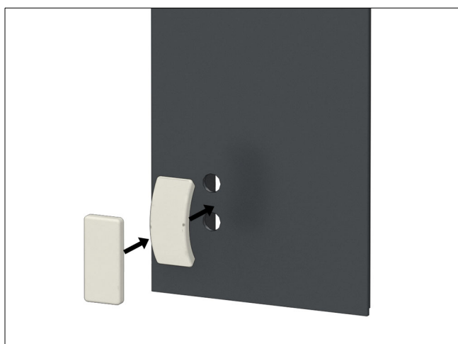
Figure 89 Flex the bumper and insert in bottom of jamb cover
