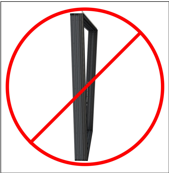
Figure 61 Make sure the entire frame is on the same plane and not twisted.
