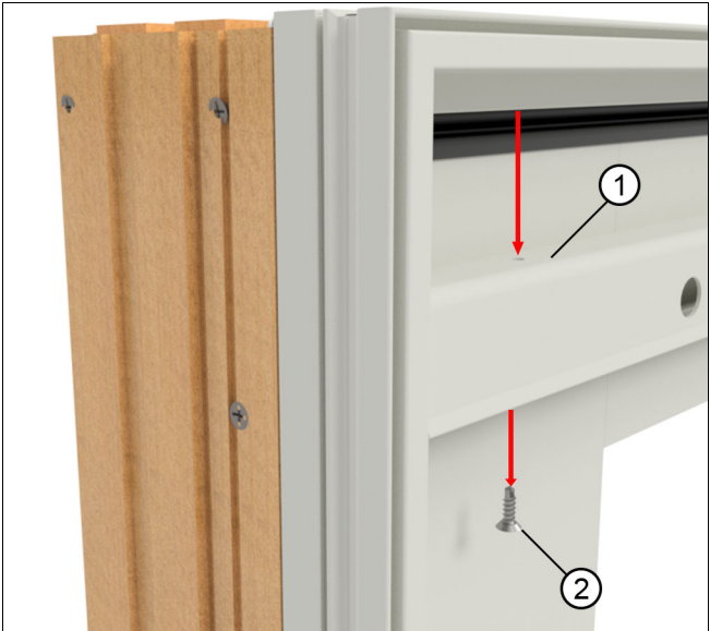
Figure 31 Remove the head jamb screen track
