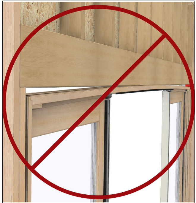
Figure 46 Do not bow the head jamb by over-tightening screws. (operator panels removed in this image for illustrative purposes)
