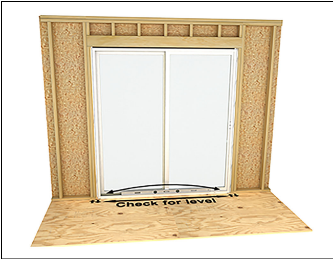
Figure 4 Start with a clean flat sill
